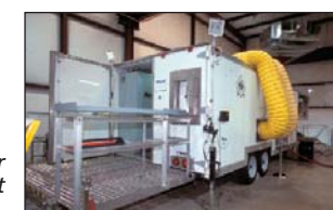
The RRS operations trailer vents air through carbon filters, protecting against an accidental vapor release.
