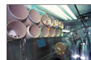
The RRS glove box station allows operators to safely unpack, sort and neutralize CAIS items and to handle and package contaminated solid waste associated with CAIS.
