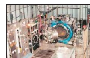
The EDS containment vessel is resistant to corrosion, allowing it to treat a wide variety of munitions.
